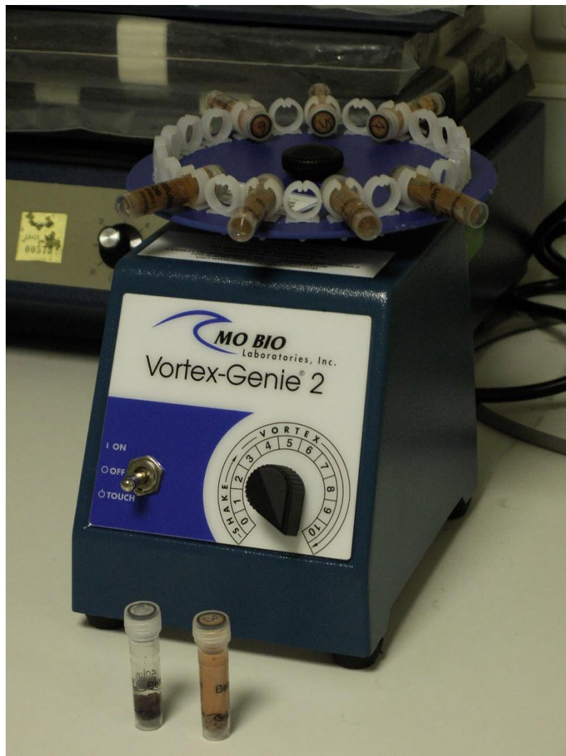
Figure 69- Vortex-Genie 2 Vortex and the fitted vortex adaptor. The platform has been designed specifically for vigorous mixing and homogenization of multiple samples simultaneously.
