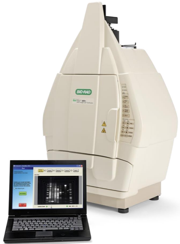
Figure 84- A gel documentation system required to visualize DNA fragments (Bio-Rad 2017).
