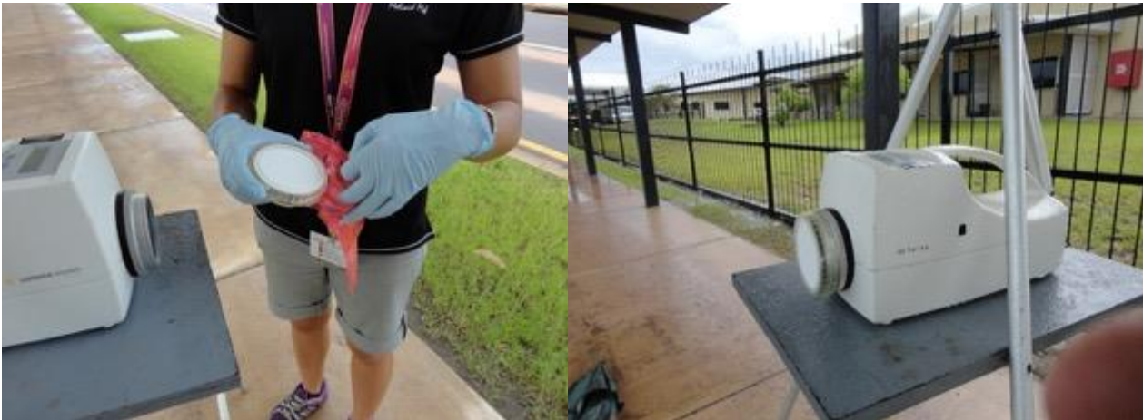
Figure 23- Air sampling for B. pseudomallei using portable electric filtration device (Sartorius MD8 Air Sampler) and disposable gelatine membrane filters (Sartorius 80mm) (Images courtesy of Menzies School of Health Research, Australia).
